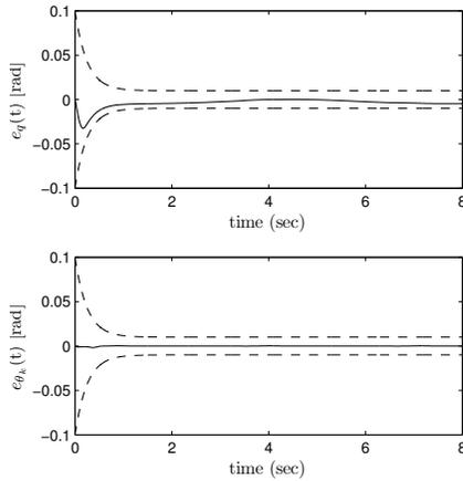
Fig. 6: Output errors (solid lines) along with performance bounds (dashed lines).
