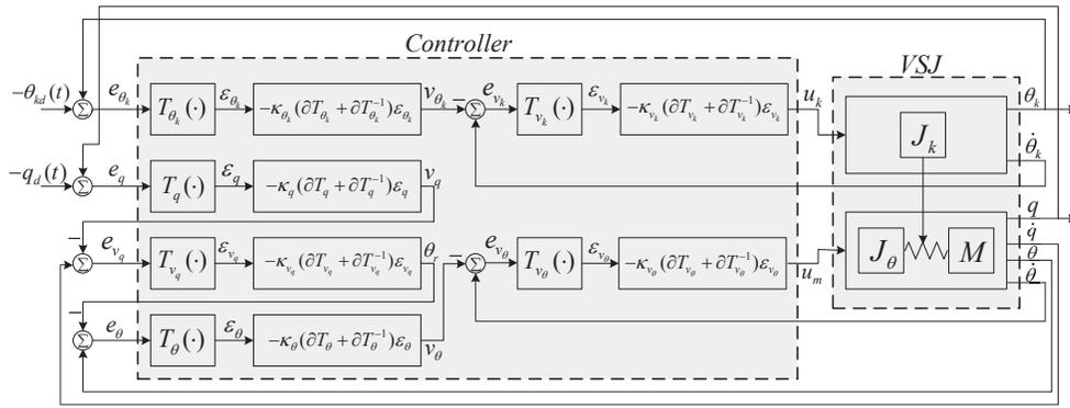
Fig. 4: The proposed control scheme.
